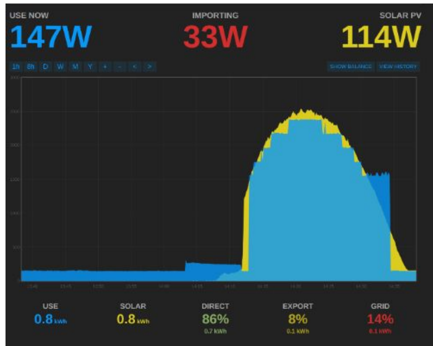
OpenEVSE solar PV diversion example. Yellow: solar PV, blue: OpenEVSE.
